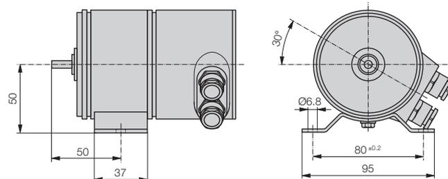
Fig. 13. Fixing with mounting foot.
