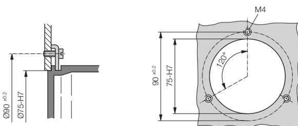
Fig. 12. Left: Fixing with clamps
