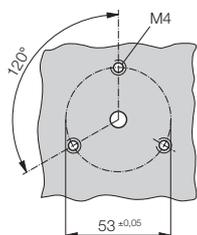
Fig. 10. Drilling plan for measuring instrument housing.
