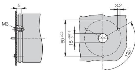
Fig. 8. Left: Fixing with cheesehead screws
