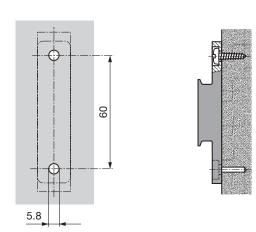
Fig. 5. Drilling pattern.
