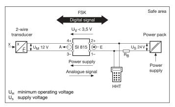
Fig. 10. SINEAX SI 815-5111. Standard (non-Ex) version, designed for FSK communication, frequency 500 Hz ... 35 kHz.
