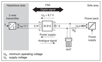
Fig. 11. SINEAX SI 815-5.11. Ex version, (output signal A "intrinsically safe"), designed for FSK communication, frequency 500 Hz ... 35 kHz.
