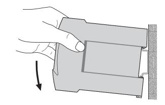
Fig. 4. Mounting on top-hat rails  $35 \times 15$  or  $35 \times 7.5$  mm.
