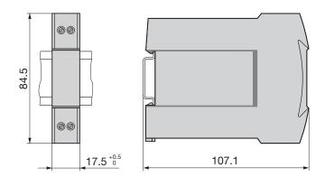
Fig. 14. SINEAX SI 815-5.... (housing **N17**) clipped onto a top-hat rail (35  $\times$  7.5 or 35  $\times$  15 mm, acc. to EN 50 022).
