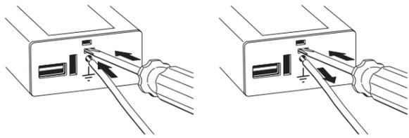
Fig. 8. Connect the earth connection to the PK 610 interface.
