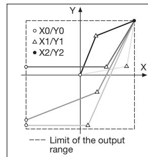
Fig. 11. Examples of settings with bent characteristics.
