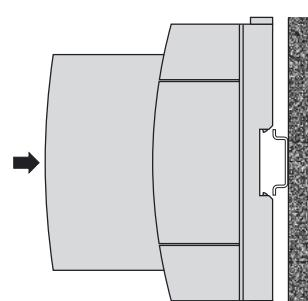
Fig. 5. Mounting on top-hat rail
