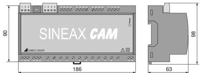
SINEAX CAM in DIN-rail behuizing (35 x 15 mm of 35 x 7,5 mm).
