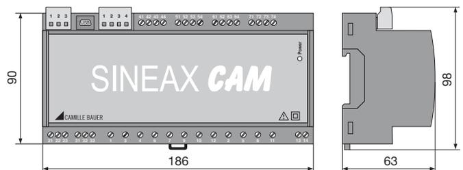
SINEAX CAM in mounting rail housing snapped on top-hat rail (35 x 15 mm or 35 x 7.5 mm). Terminals partly pluggable.
